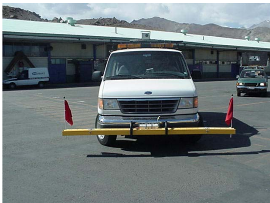
Figura 1.3. Transverse Profile Logger (TPL)
