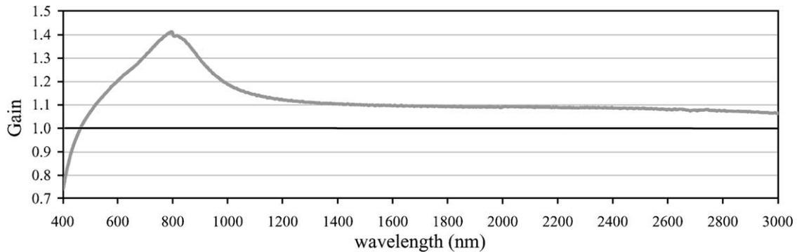
Fig. 1. Gain offered by our 4-layer protected Ag over Al for a 3-mirror telescope.
