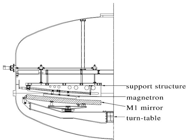
Fig. 2. Cross-section of the vacuum chamber.
