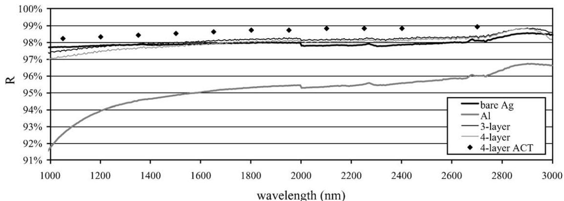
Fig. 4. Comparison of Al, bare Ag and protected Ag in the NIR (data with Cary 5 at ODA).
