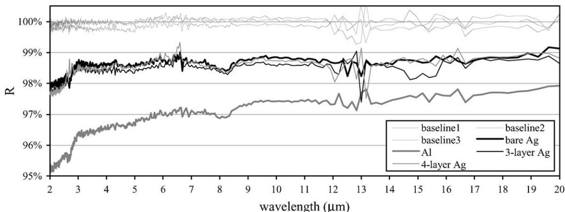
Fig. 5. Comparison of Al, bare Ag and protected Ag in the MIR (data with PE983 at ODA).
