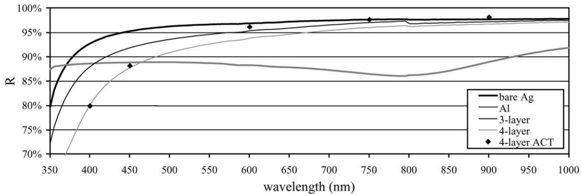
Fig. 3. Comparison of Al, bare Ag and protected Ag in the visible (data with Cary 5 at ODA).
