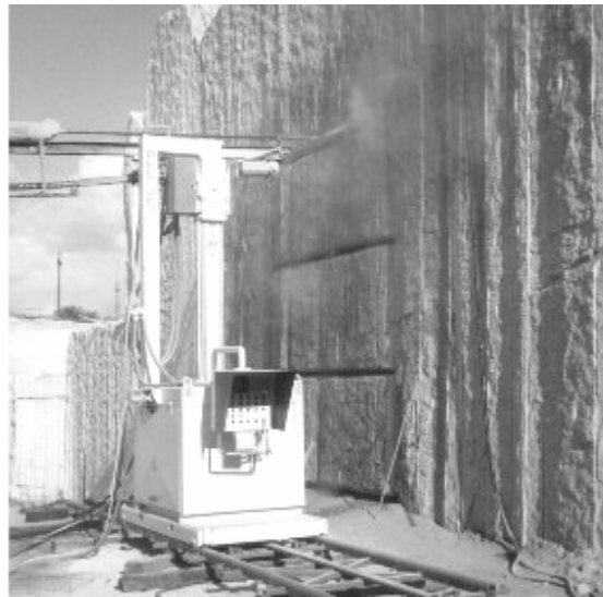
Figure 6. Waterjet slotting in a granite quarry, Sardinia.
