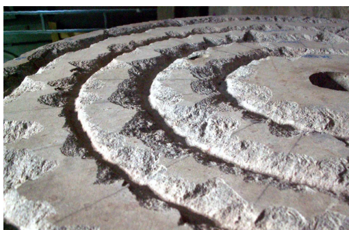
Figure 5. The concept of waterjet assisted mechanical excavation of rocks
