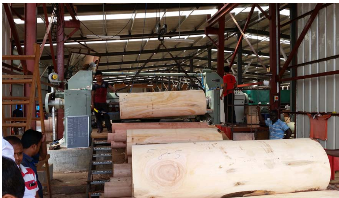
A-peeling: Logs are peeled to produce veneer in a mill in ZES Nkok, Gabon. Photo: B. Cassagne/FRM Group
