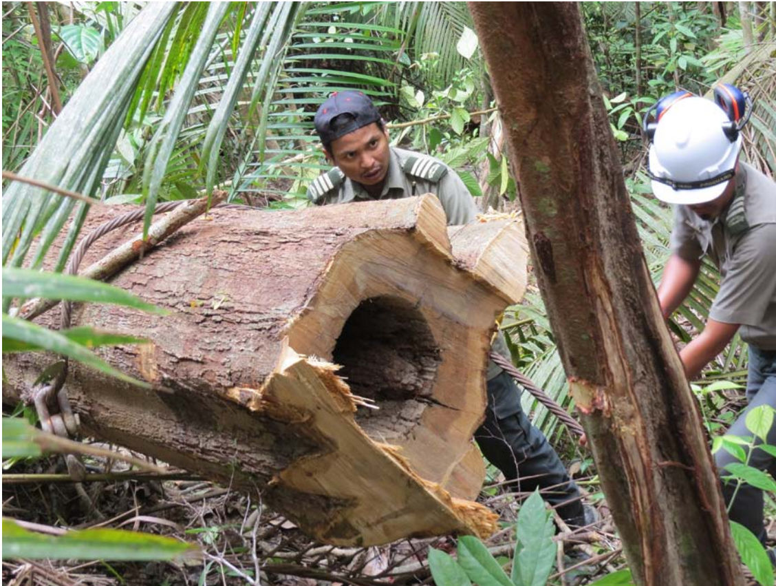
Haulage: Workers attach a choker to a log as part of the extraction process. Photo: A. Khalim/Forestry Department Peninsular Malaysia
