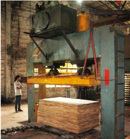
Flat pack: Plywood panels are pressed in a factory in Hainan Province, China. Photo: J.-C. Claudon/ITTO
