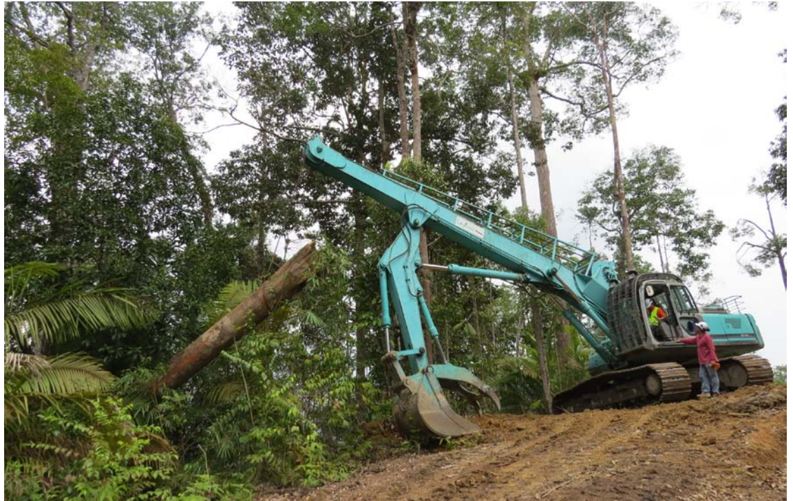
Long reach: A “logfisher” machine extracts a log to a landing in hill forest in Peninsular Malaysia as part of a demonstration of reduced impact logging. Photo: A. Khalim/Forestry Department Peninsular Malaysia
